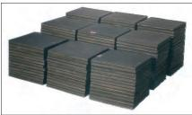
Scientifically designed resilient pads are moulded with high grade blend of Natural and Synthetic Rubber for general applications. The pad surfaces on both sides have moulded recessed offset-cells to allow flow of rubber when under load while maintaining lateral stability. This design eliminates the shape factor usually associated with elastomeric pads and provides positive grip to machine foot and foundation when under load.
