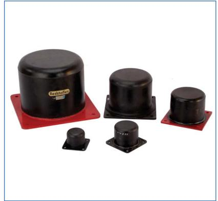
If one Buffer displays insufficient energy absorption characteristics, 2 units can be connected in series, one being attached to the moving part of the machine and the other to the fixed part. Double energy absorption is thereby obtained.
